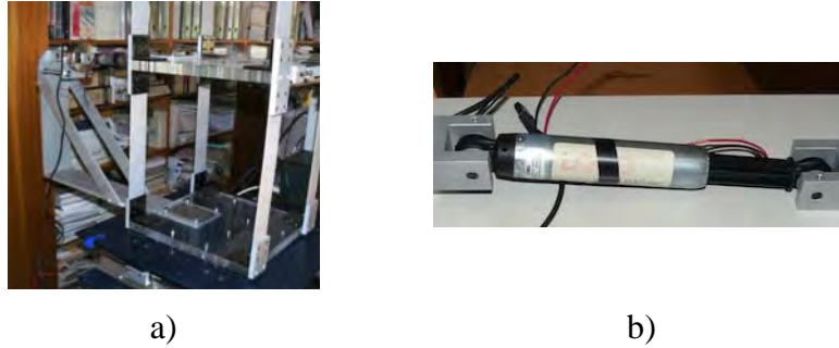
Figure 4: a) MR damper attached to the experimental metallic frame; b) RD-1097-01 MR Damper.
