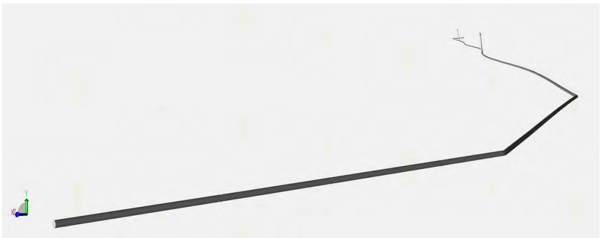
Figure 5: Caesar II representation of the fourth mode shape driven by the ASCE-7 spectra – Liquid transmission line.
