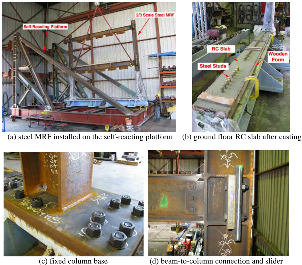
Figure 4: Erection and typical connection details of the physical subassembly part of the hybrid model.
