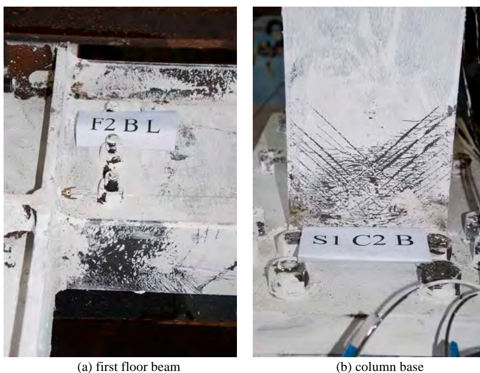
Figure 13: Structural damage observations during testing Phase I.
