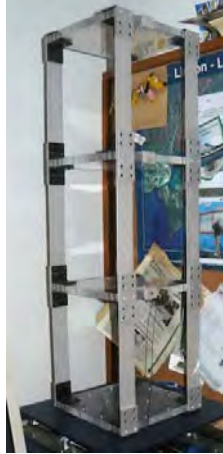
Figure 2: Metallic scaled frame at the shaking table.
