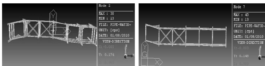
Figure 11 First two vibration modes of the pipe-rack model
