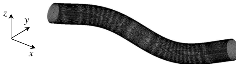
Figure 12: 3 rd flexural mode (3F, f = 1,835 Hz).
