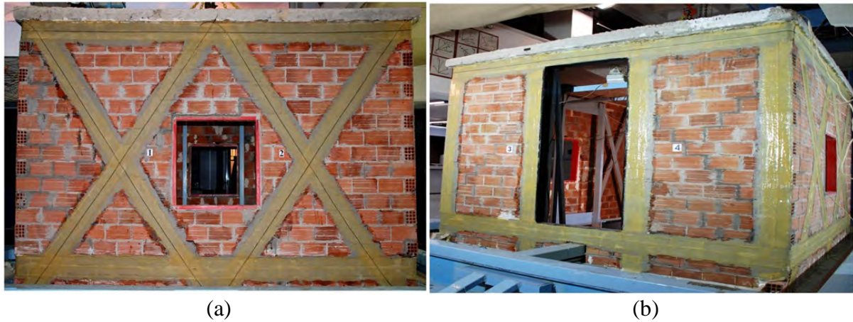
Figure 8: A picture of the repaired masonry building with reinforced GFRP strips; (a) sides 1-2, (b) sides 3-4.
