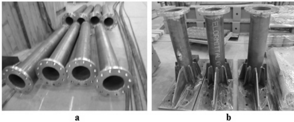
Figure 24 Test specimens for: (a) bending tests; (b) axial tests.
