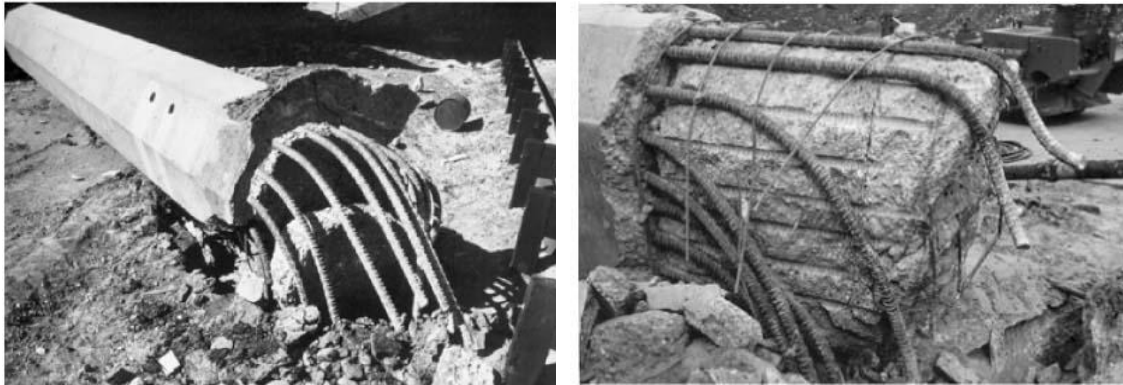
Figure 1: Pull-out of longitudinal reinforcement in bridge columns from foundations during the San Fernando (1971) earthquake [1]
