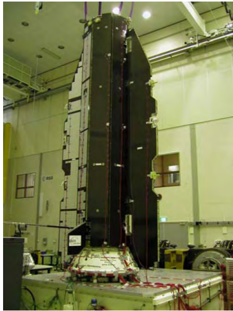
Figure 2: GOCE satellite on large slip table at ESTEC (courtesy of ESA).
