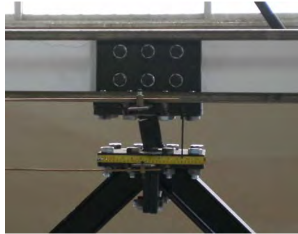
Figure 18: Failure mode of the link element (F2)
