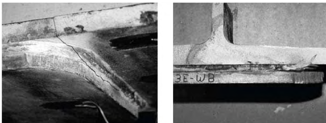
Figure 2: Examples of distortion induced fatigue crack progression [9].
