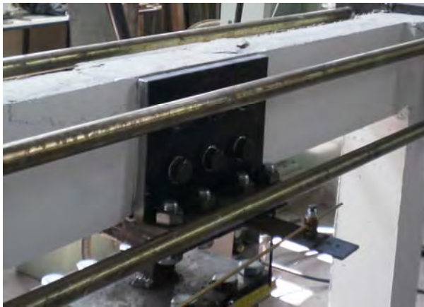
Figure 19: Concrete cover failure (F2)
