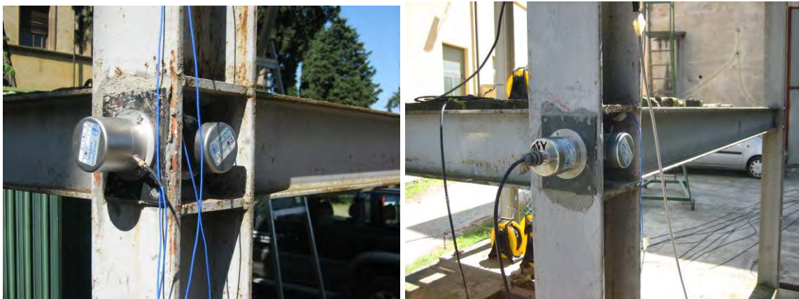
Figure 2: Accelerometers disposition (level #1).
