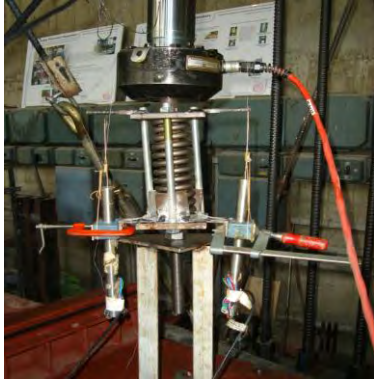
Figure 4. Test for measuring the spring stiffness
