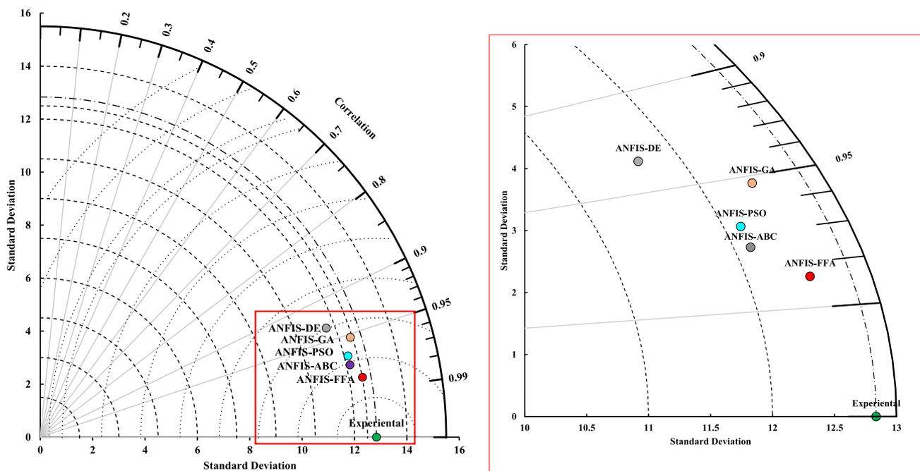
Fig. 8 Statistical comparison of the proposed hybrid models based on the ANFIS approach with the experimental values, using the Taylor diagram
