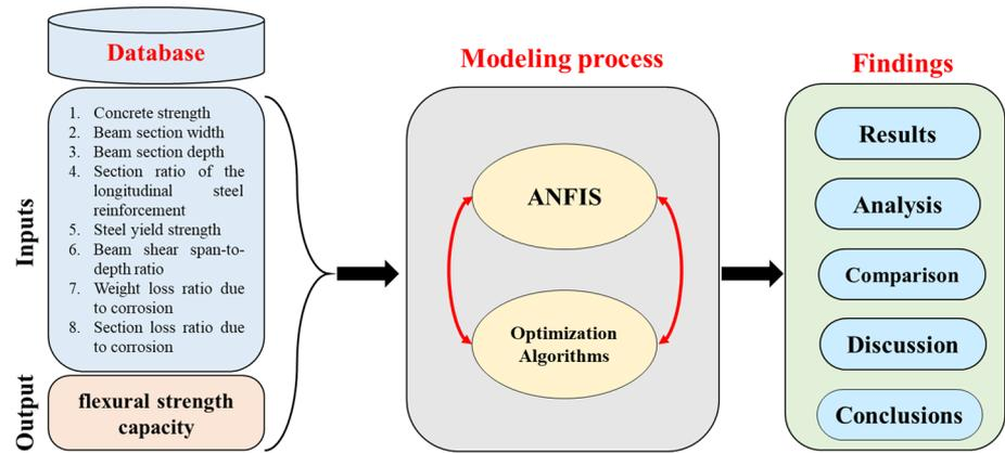
**Fig. 2** The structure of adaptive neuro-fuzzy inference system (ANFIS) technique for modeling flexural strength capacity ( $M_{fx}$ )
